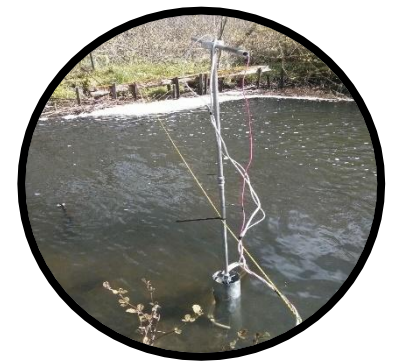
Streambed Point Velocity Probe (SBPVP)
