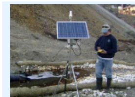
Water monitoring at the New Idria Mercury Mine Superfund site in California involves use of time-interval sampling devices powered by solar energy. Collected sampling data are transmitted via satellite to a website accessible by project staff. This approach supplies a renewable source of onsite energy and reduces the frequency of staff visits to this remote site. Ongoing investigation of this site led to removal actions in 2011 and 2015.
