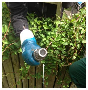
Plugging of the tip during top-down injection (settling of mZVI during transition between injection intervals). Change was made to flushing out the rods with anaerobic water before transitioning to the next lift.
